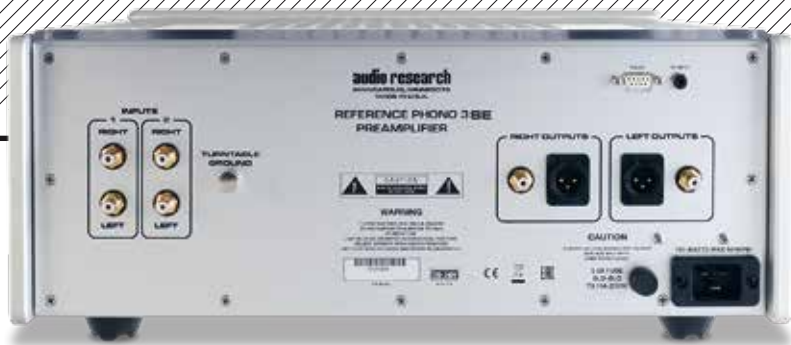
ABOVE: Two RCA inputs have independent 47kohm/50ohm-1kohm loading. Single-ended (RCA) and balanced (XLR) outs are capable of very high o/p [see Lab Report]
